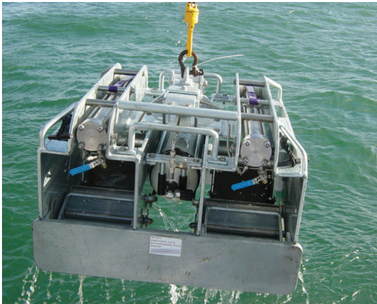
Figure 14. Costerus pneumatic twin grab (MALSF © Crown Copyright 2011).
