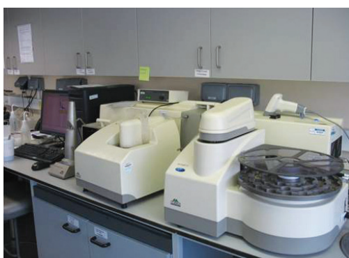
Figure 21. Malvern Mastersizer 2000 laser sizer. This equipment uses laser diffraction technology to measure particle diameters. It is most frequently used to measure the finer component (<63 \mu\text{m} ) of a sediment sample (Cefas © Crown Copyright 2011).
