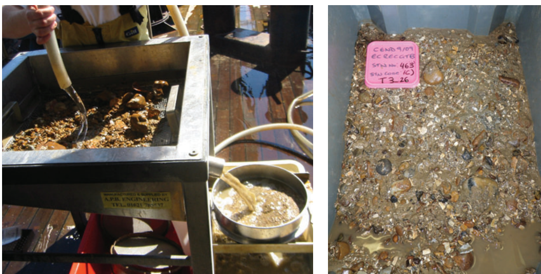
Figure 17. Labelled macrofaunal grab sample (right) awaiting processing (left) using a purpose built sieving table. The sample is being washed over a 5 mm square mesh aperture sieve supported by a removable square stainless steel frame. Note also the 1 mm mesh sieve held within a sieve holder beneath the outlet pipe of the table (Cefas © Crown Copyright 2011).
