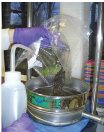
Figure 20. The automated wet sieve shaker is used to split a sediment sample into a coarse fraction and fine fraction. The coarse fraction remains on the sieve, and the fine fraction passes through the sieve to be retained in a collecting pan. The two fractions may then be treated separately for further particle size analysis (Cefas © Crown Copyright 2011).
